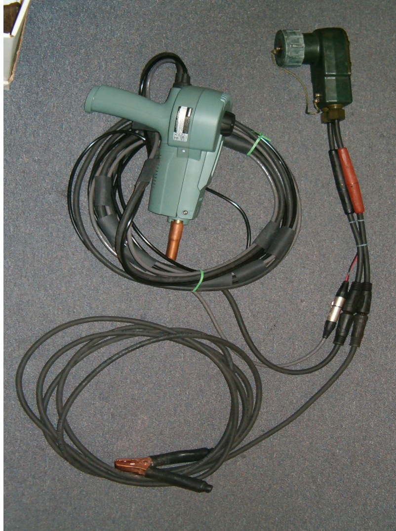
GOWELD setup with Slave Plug (600143) and Slave Plug Adapter Wiring Harness (600158). Note GOWELD is shown with Straight polarity (electrode negative) for field welding with flux-core wire.
